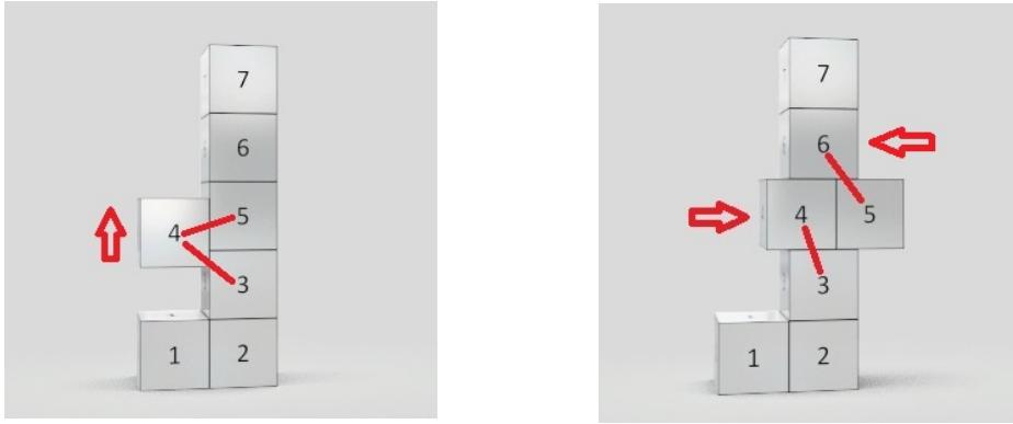
Figure 10. Snapshots from animated simulation of a self-configurable column
